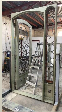
Door & Components Assembly/Inspection
